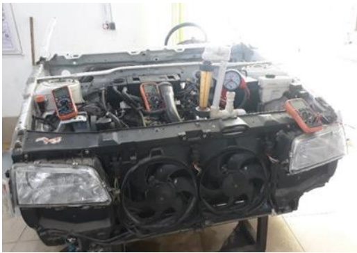
Figure 8: Measuring equipment installed on the XU7 engine
